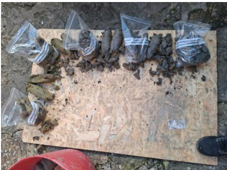
BH01 samples bagged
