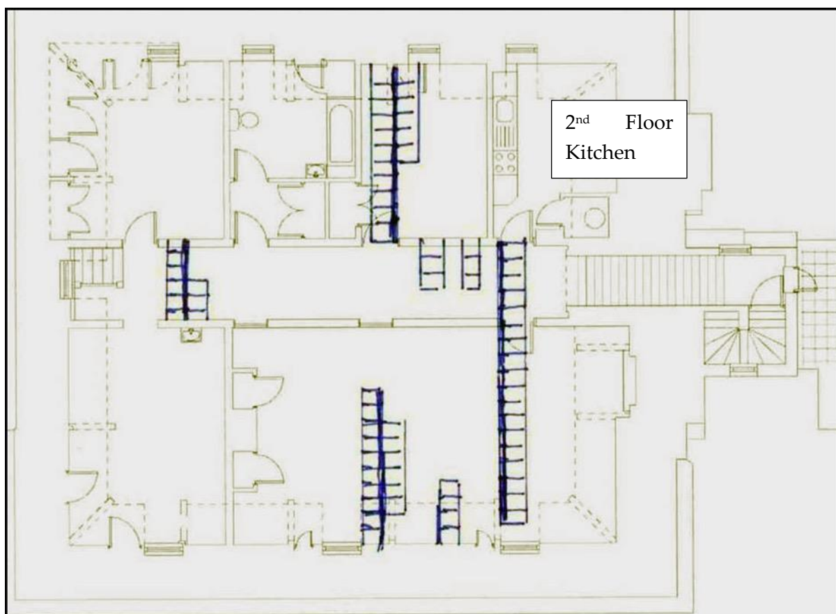
Fig 1: Mompesson 2 nd Floor- Floorboards lifted and exposed structure from CCW 2012 Survey Report.
