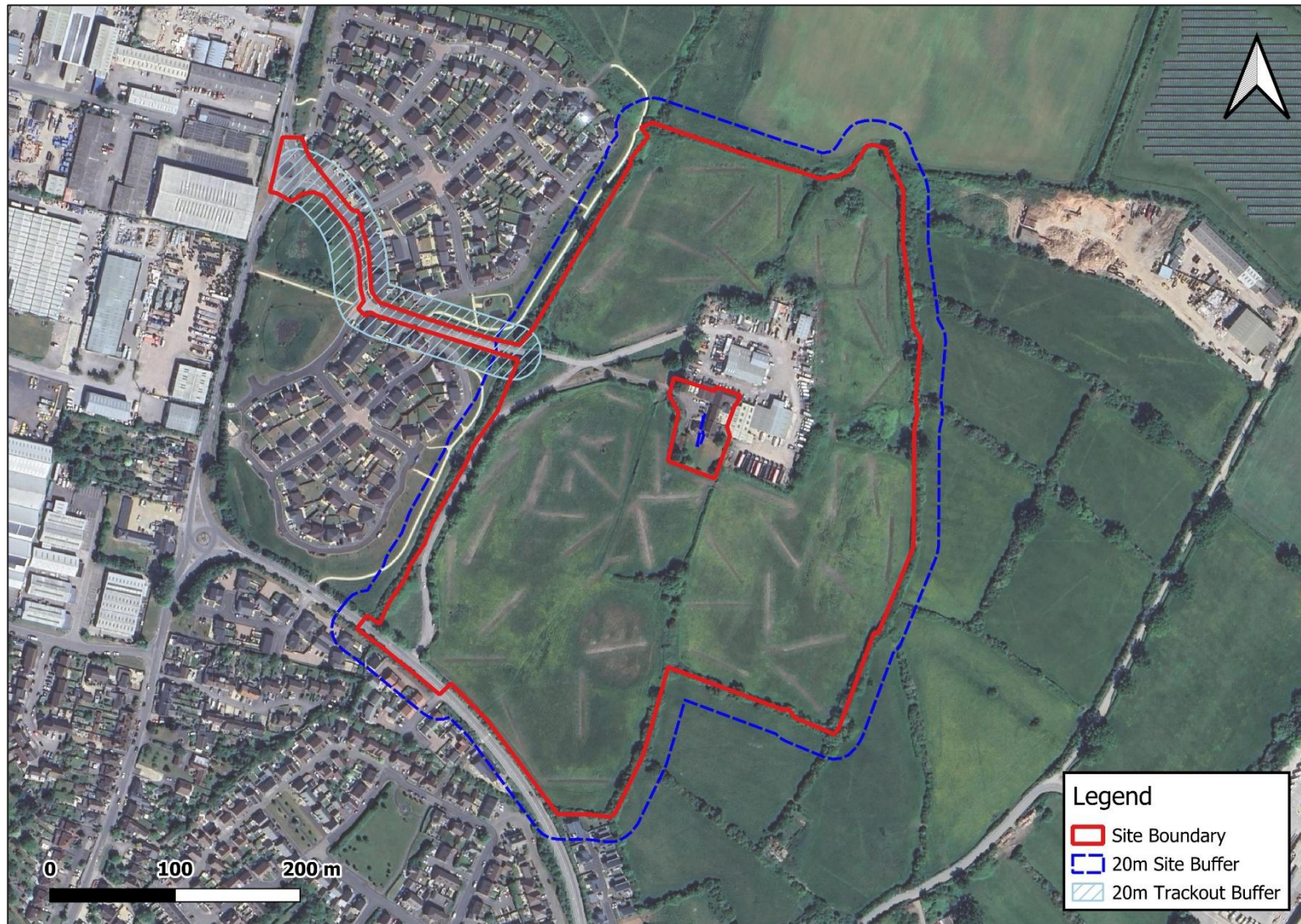
Figure 5-1: Construction Dust Buffers
