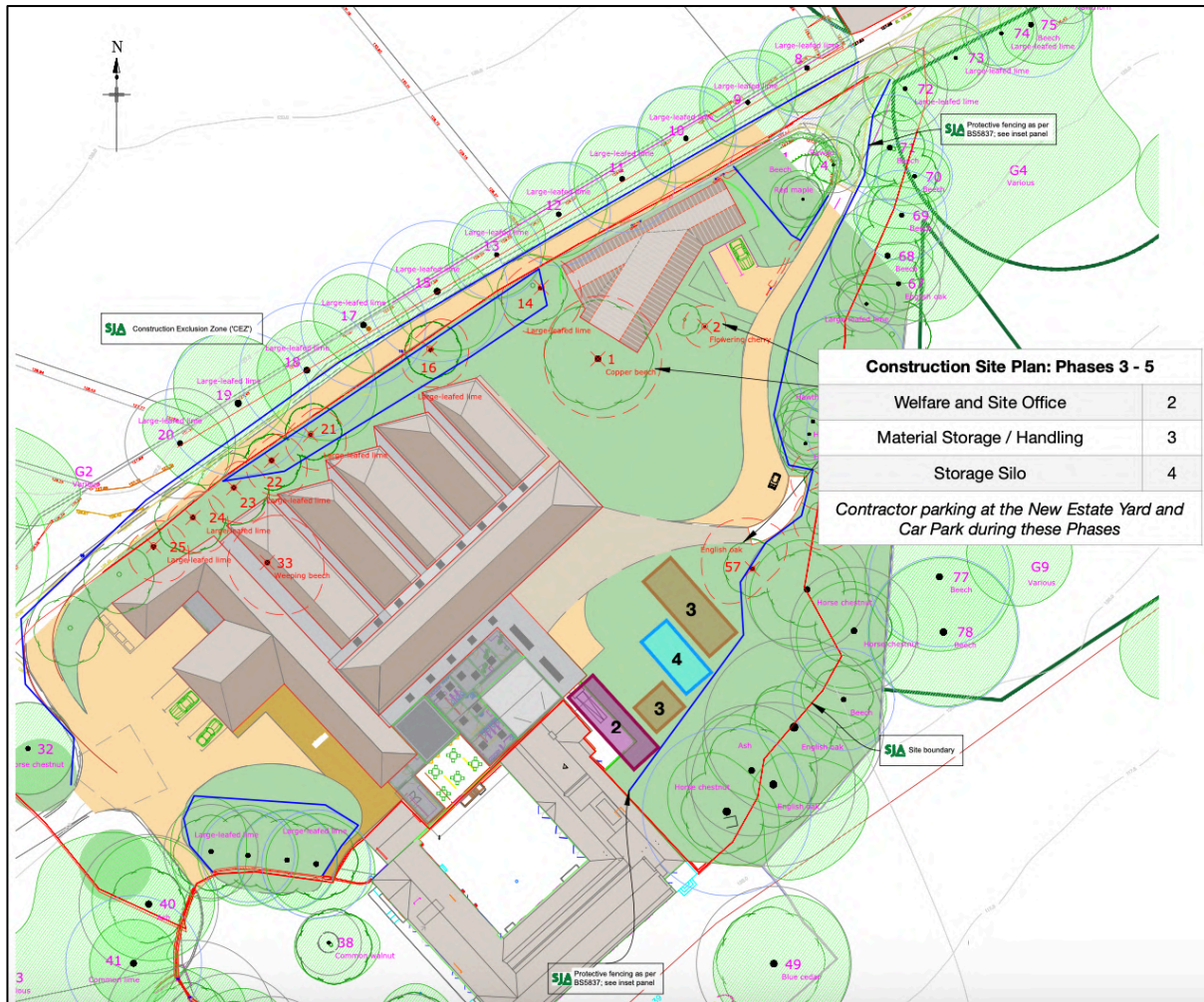
Figure 5 – Construction Site Plan: Phases 3 - 5
