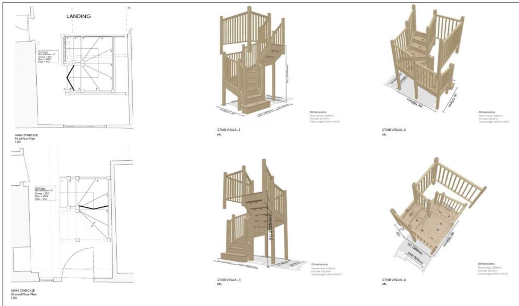
Fig. 27: Plans and construction details for the proposed new main staircase (Ben Lilley Design Studio).
