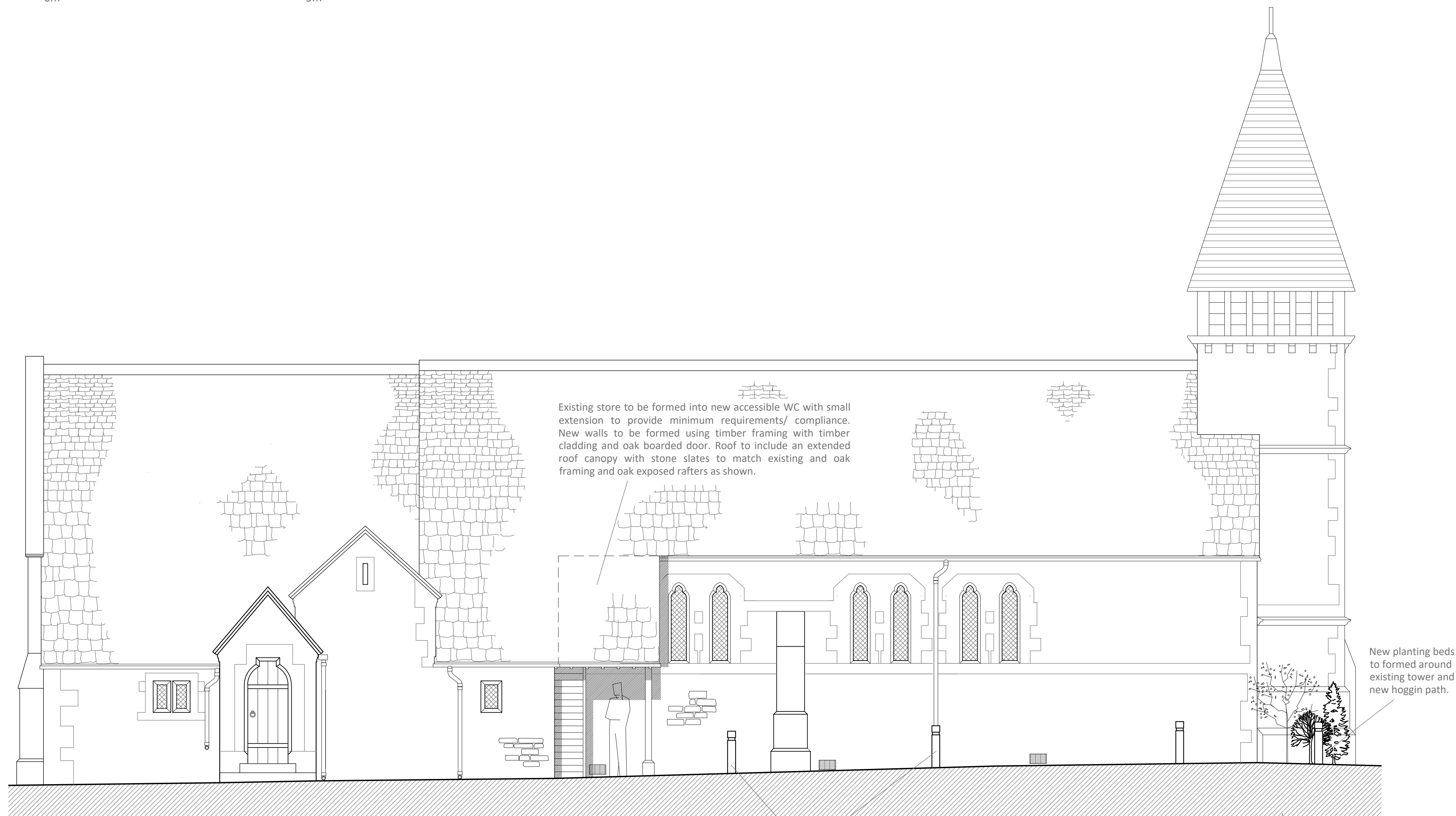
North Elevation As Proposed - Scale 1:50
