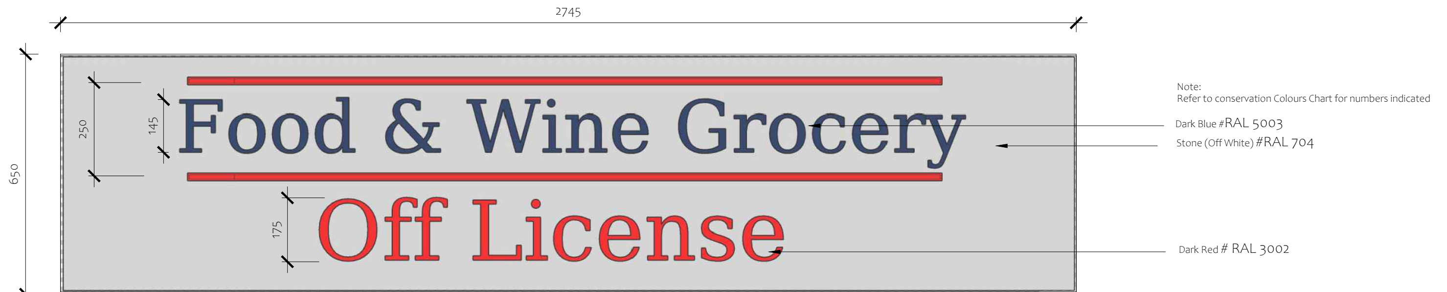
Bays 02 & 04 (ref.EL-01) Hand Painted Sign on Backing Board
