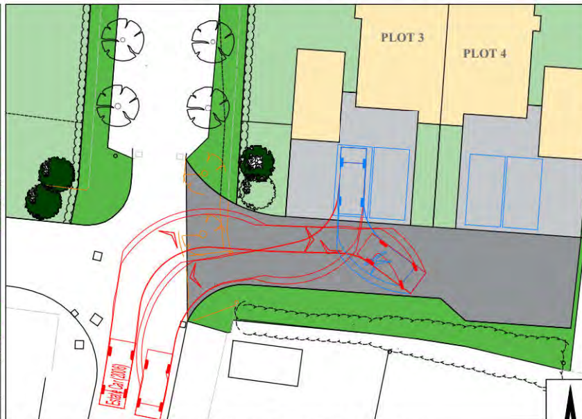
Car entering and exiting Plot 3 parking space
