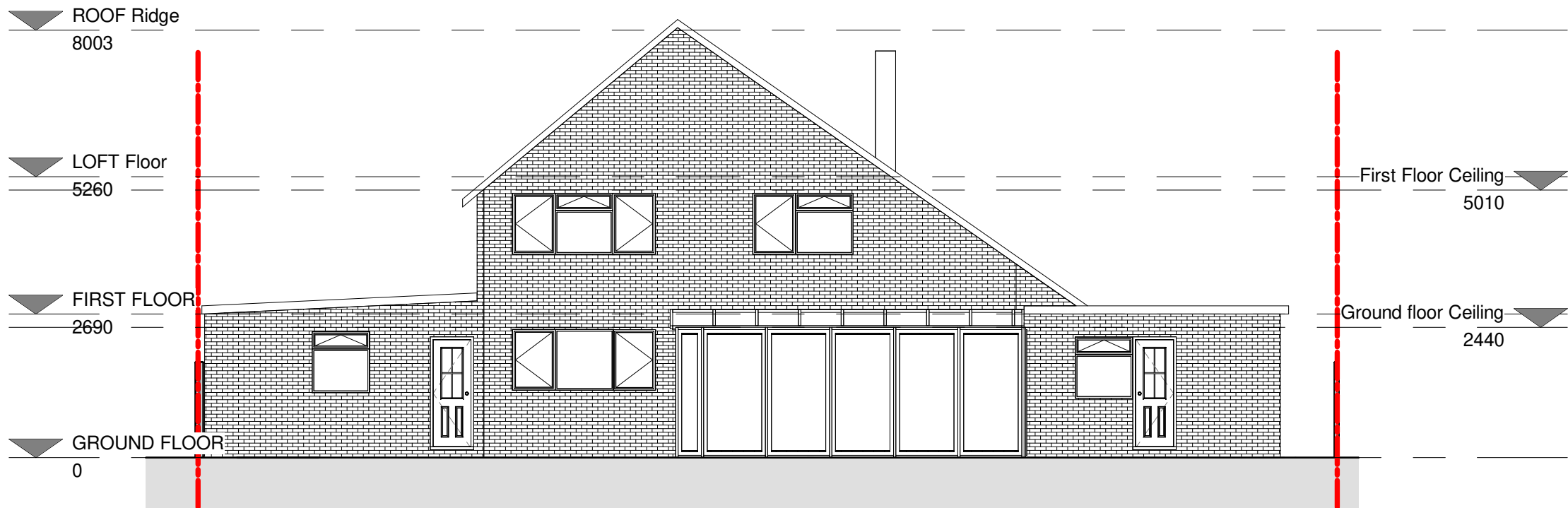
1 EXISTING REAR ELEVATION 1 : 100
