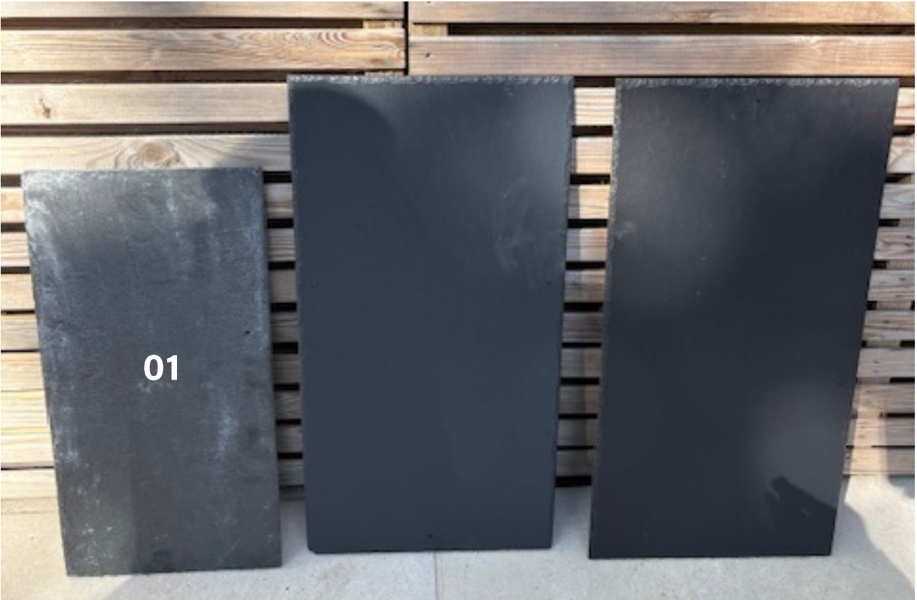
HOUSE 1 MATERIALS - roofing Natural Slate (01)
