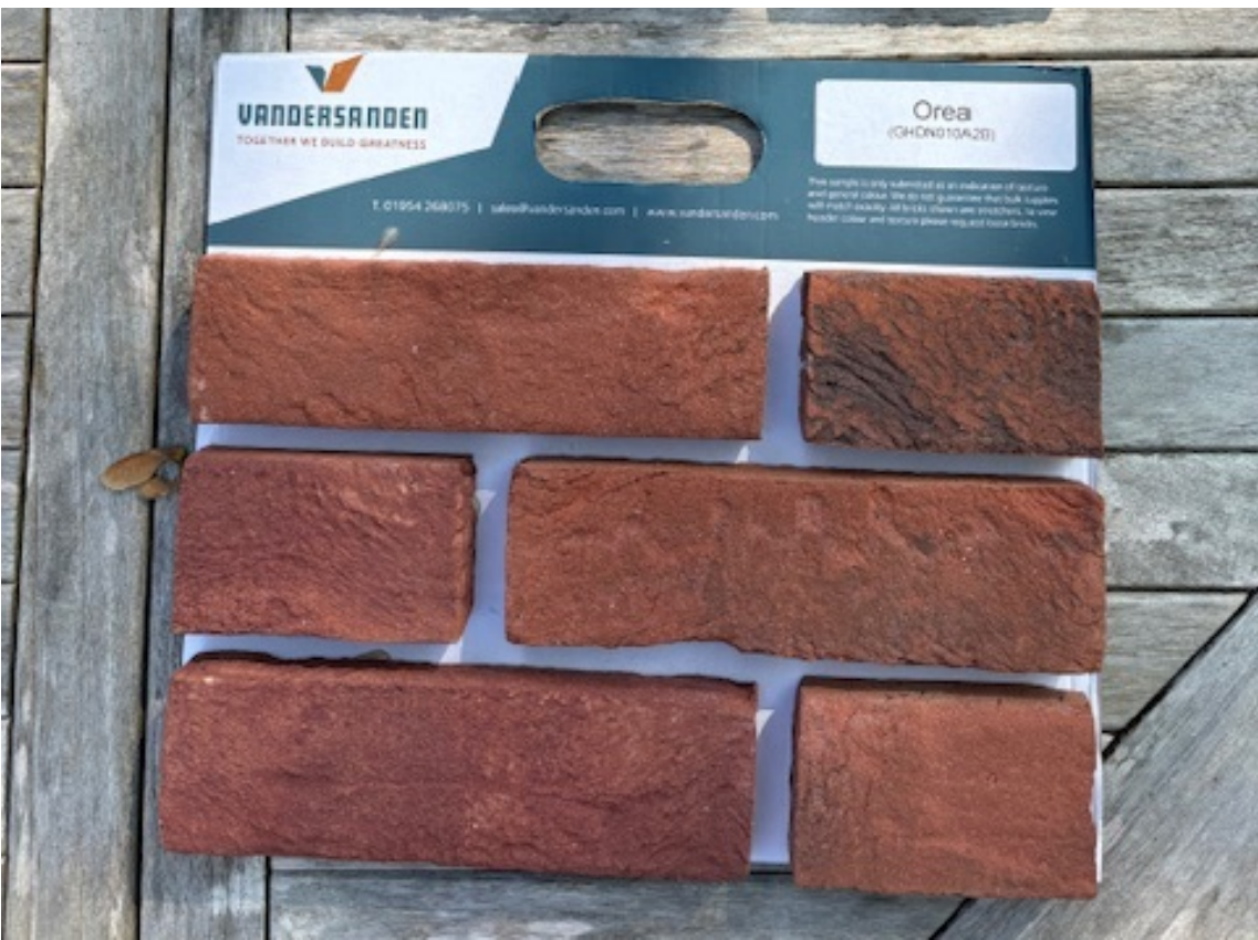
HOUSE 1 MATERIALS - proposed brickwork Vandersanden Orea - stretcher bond to main facing brickwork
