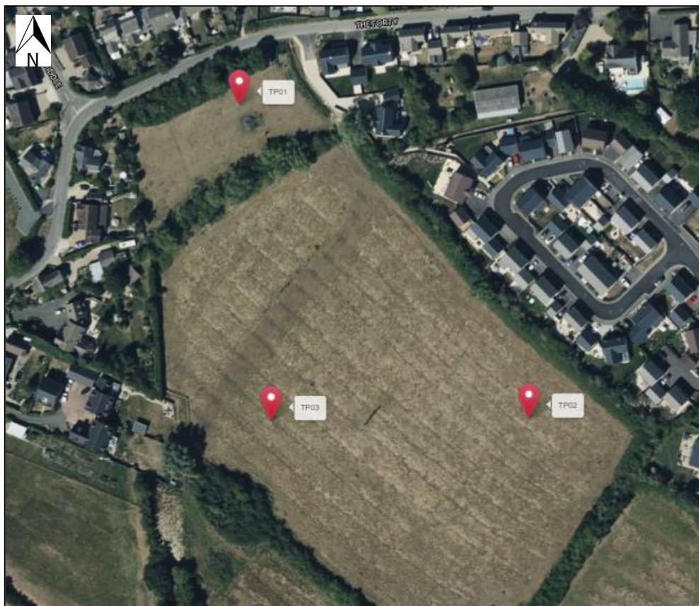
Figure 1 – Soakaway Test Location Plan
