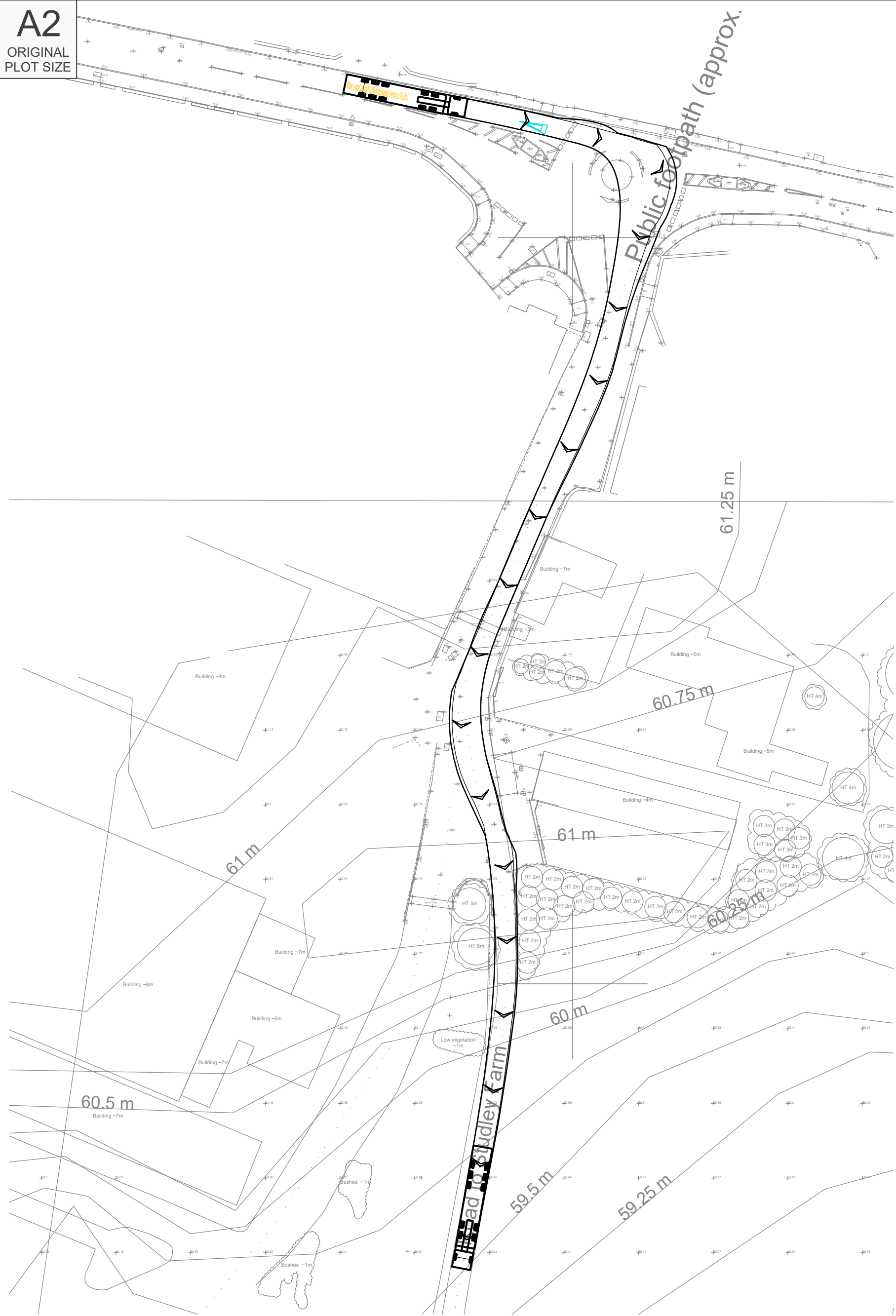
16.5m Articulated HGV Driving To Site
