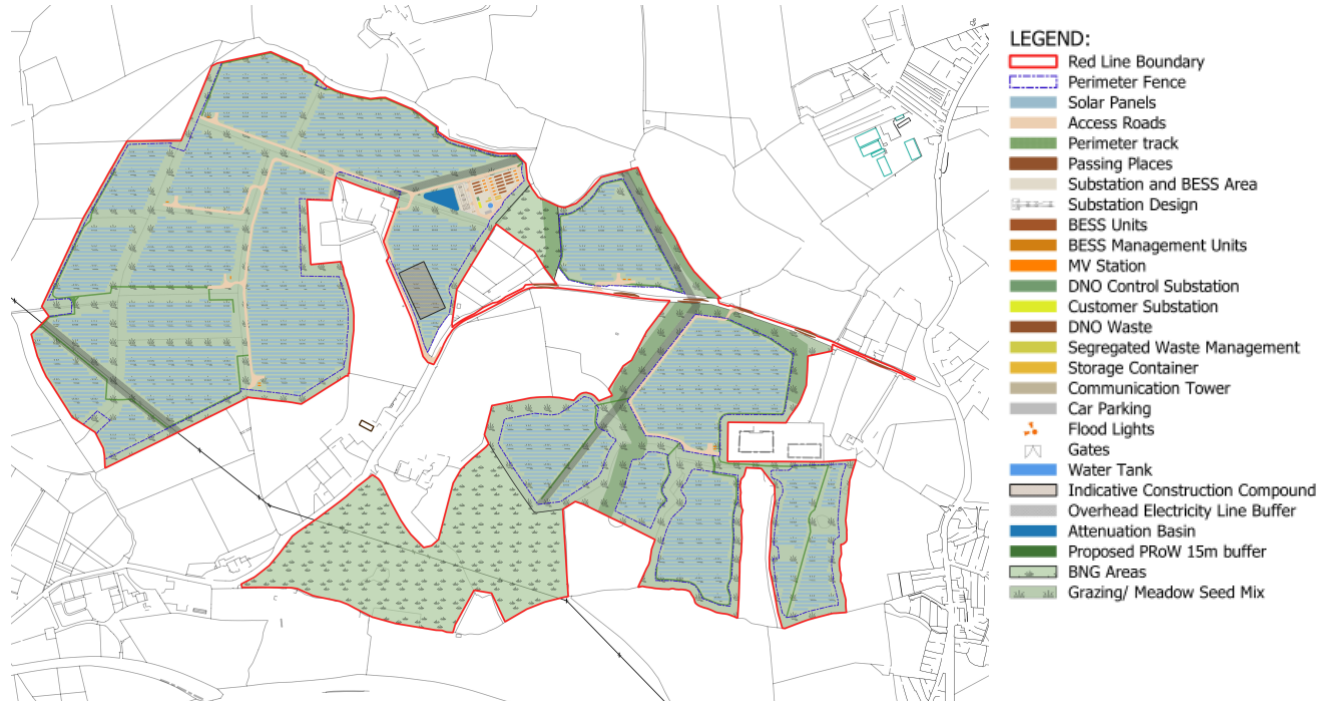
Figure 1: Flaxlands Solar Farm Proposed Layout (Ampyr Solar Europe, revision R11)
