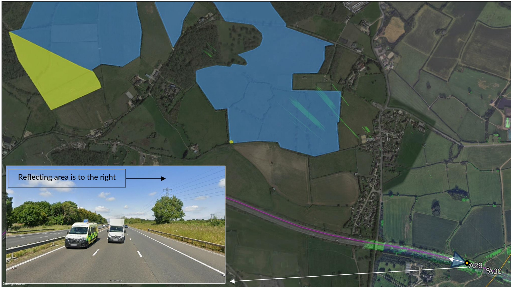
Figure 11 Reflecting panels and screening for road receptors A29 and A30, with representative ZTV viewshed and Streetview imagery from A29
