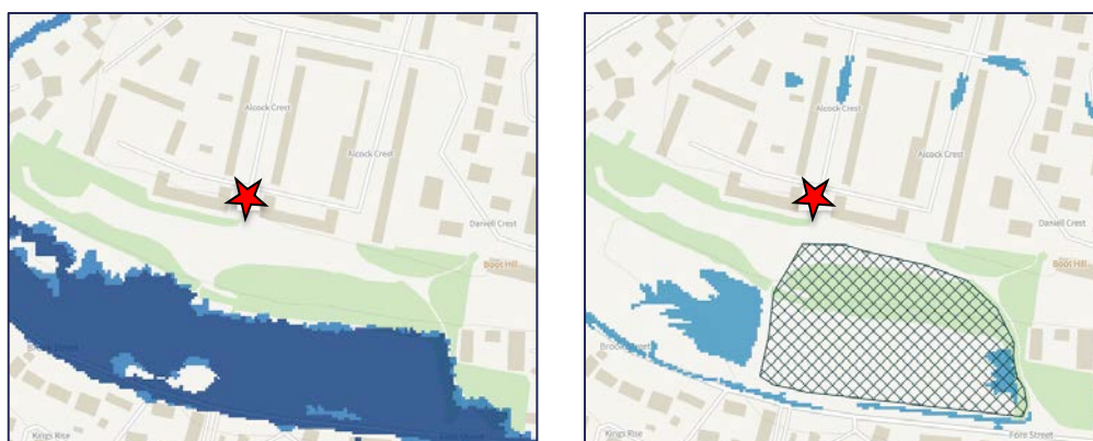
Fig. 9 Extracts from the Government's Flood Map for Planning showing the location of the site (red star) in relation to Flood Zones 2 and 3 (dark blue shading in the image to the left), and surface water flooding and flood storage (light blue shading and hatching in the image to the right).
