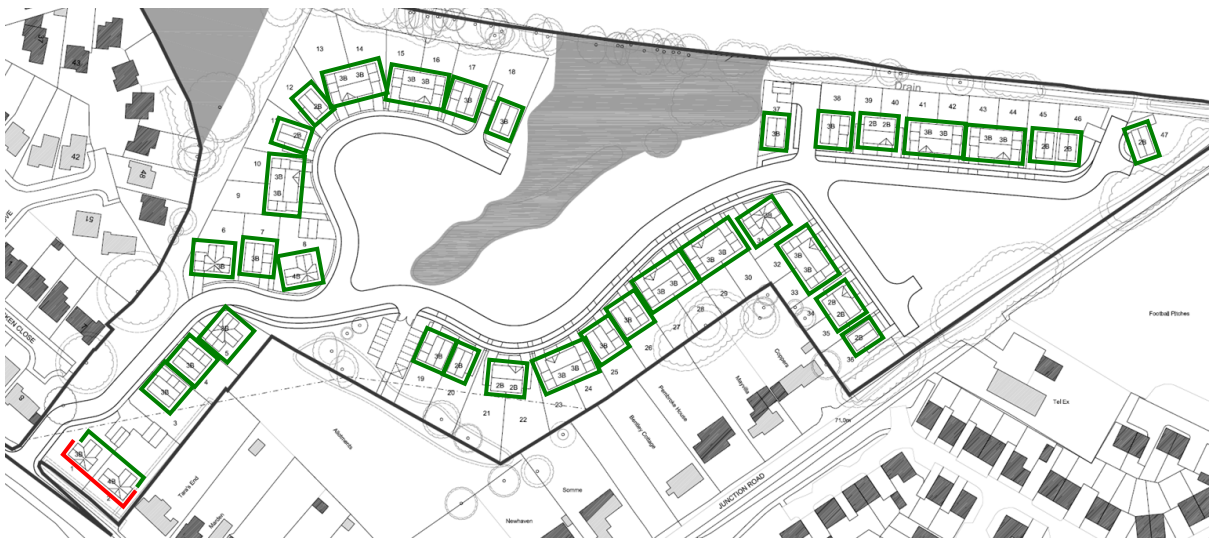
Façade acoustic specification zones (all levels)
