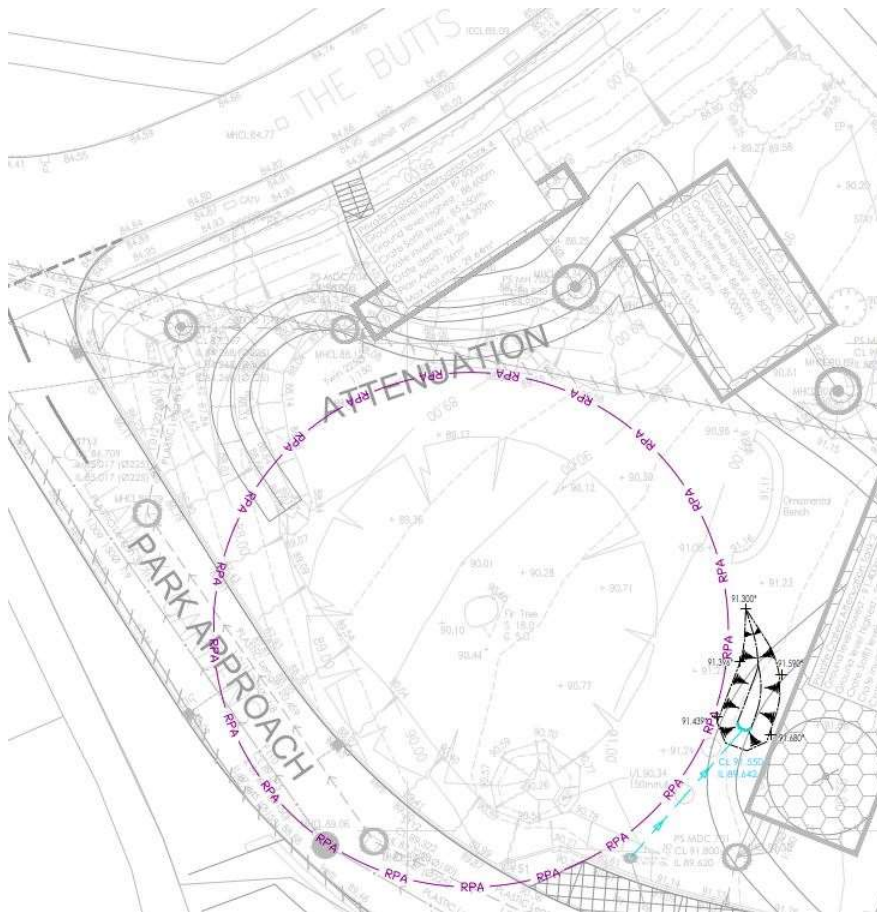
Figure 3.1 – Headwall relocation design proposal
