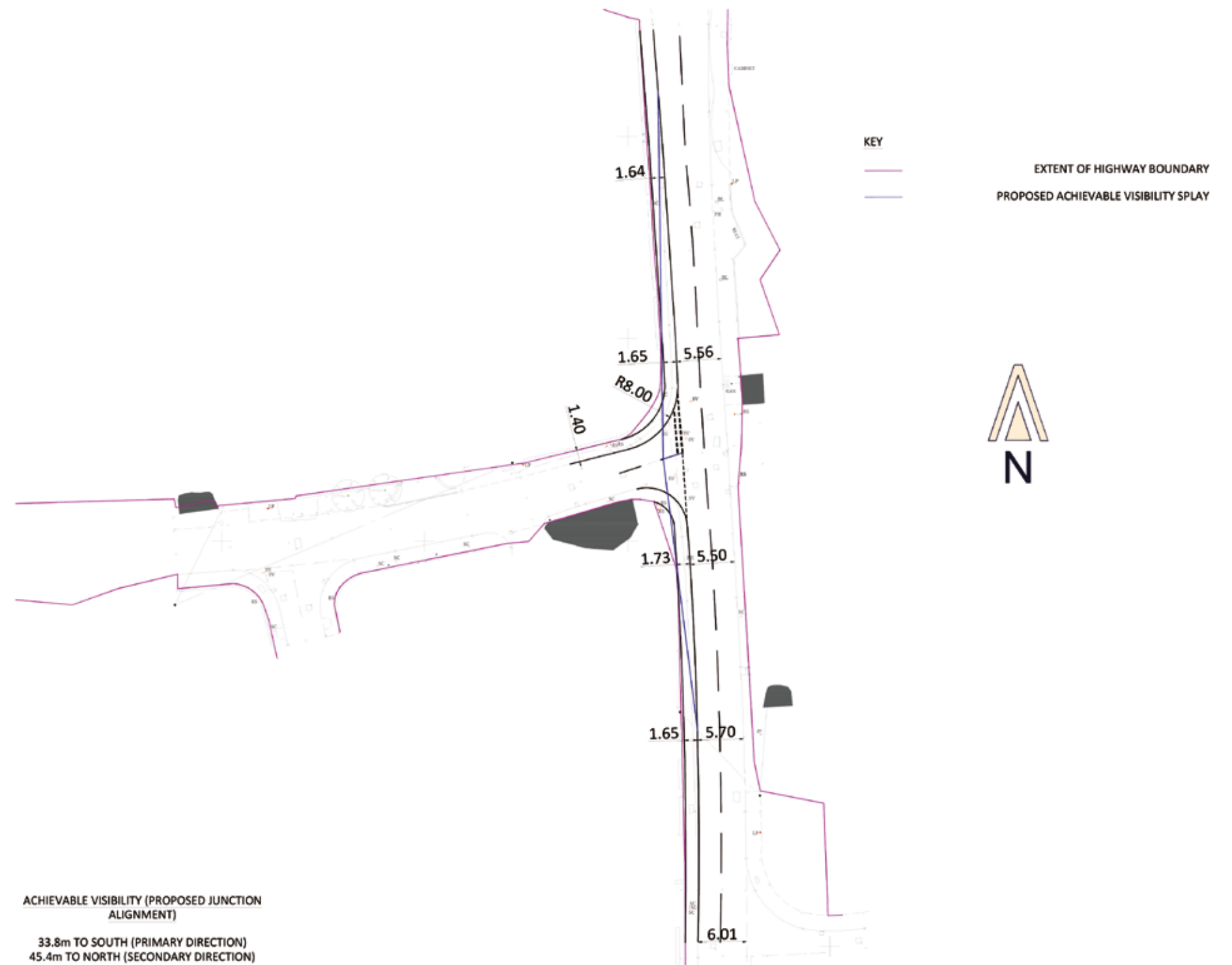
POTENTIAL JUNCTION ALIGNMENT
