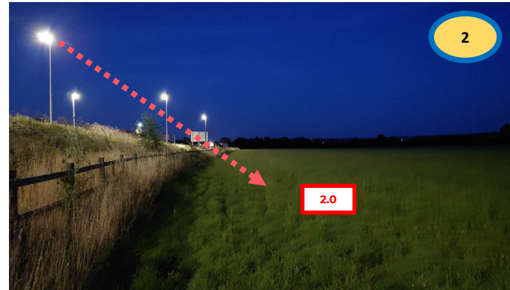
View from the northwest boundary fence looking east towards the M4 slip road and the dark east boundary hedgerow. 1.8-2.0 LUX falls into the site from the 4000k 12m tall slip road lighting.
