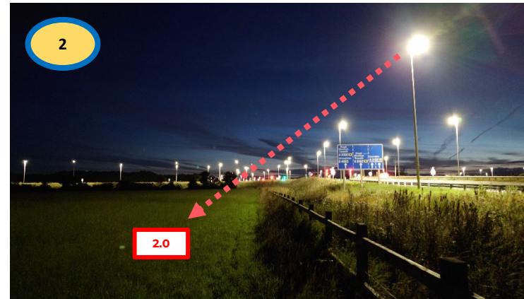
View from the north boundary fence looking west towards the M4 slip road and Junction 16. An average of 1.8-2.0 LUX falls into the site from the 4000k 12m tall slip road lighting.
