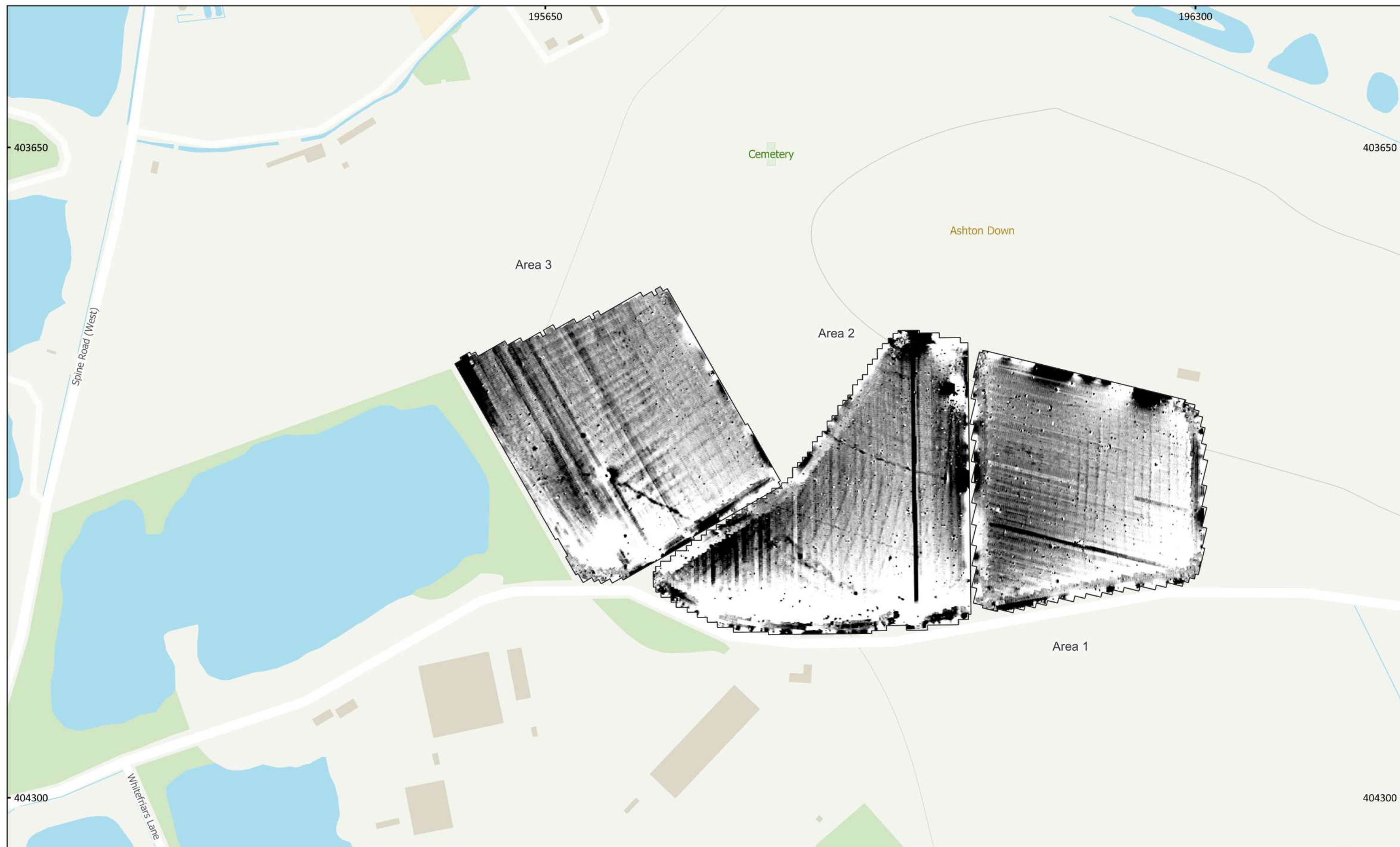
MSSU1377: Ashton Keynes, Wiltshire Figure 3 - Magnetic Total Field (Lower Sensor) (Overview) (Areas 1, 2 & 3) 1:3,500 @ A3 Copyright Magnitude Surveys Ltd 2022 Contains Ordnance Survey data © Crown Copyright and database right 2022
